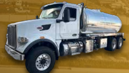
2025 PETERBILT 567 , CUMMINS ISX 450 HP, ALLISON 4500 RDS AUTO. TRANSMISSION, 4200 ALUMINUM TANK, NVE 4310 BLOWER 940 CFM, 36" TOOLBOX, CHROME PACKAGE, 66 GVWR. PRICE $286K + FET
