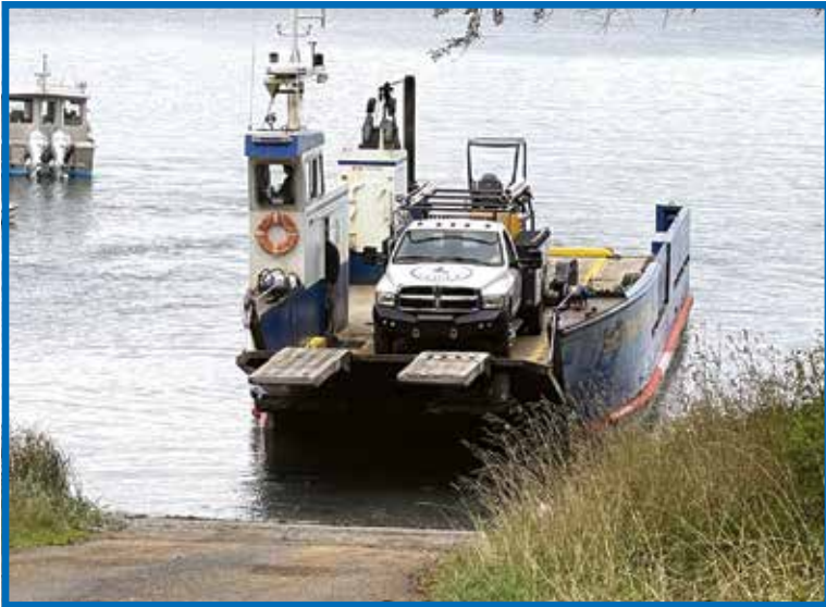
Heading out to service the outer islands with a 2005 Ram 3500 built out by Erickson with a 400-gallon aluminum tank and Masport pump.
