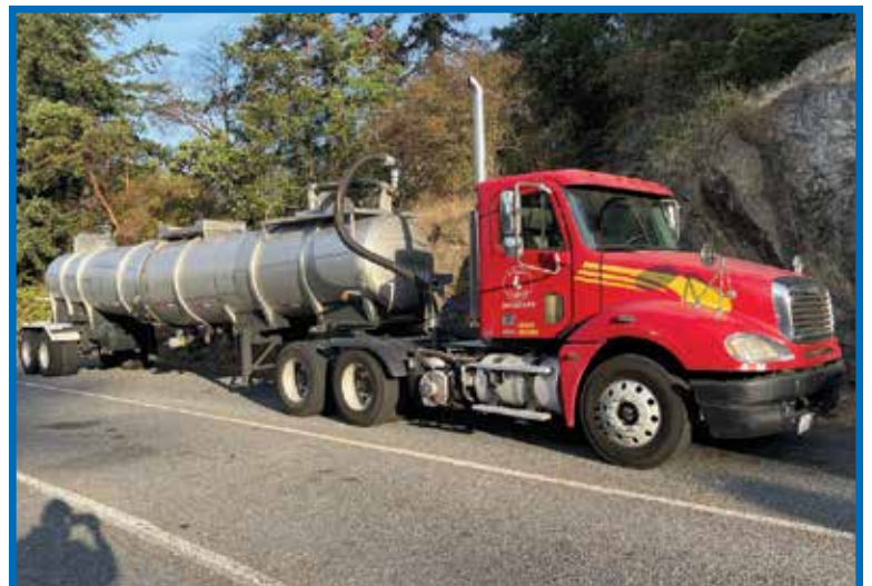
A 1989 Freightliner from Erickson Tank & Pump with a 6,000-gallon stainless steel tank and Masport Cobra pump used to transport collected waste to an off-island disposal site. (Photos courtesy of Jason Kramer)
