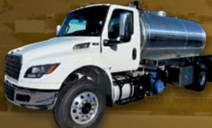
2025 INTERNATIONAL MV607 , CUMMINS ISB 300 HP, ALLISON 3000 RDS AT, AIR RIDE SUSPENSION, 2500 ALUMINUM TANK, FRUITLAND RCF 500 VACUUM PUMP, 24" ALUM. TOOLBOX, 33K GVWR. PRICE $161K
