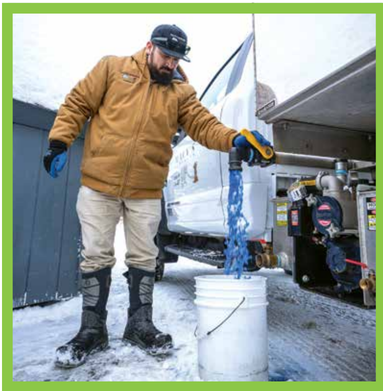
▲ Technician Juarez pours holding tank recharge water from his service truck, a Ford F-600 built out by KeeVac Industries and running a Masport pump.
