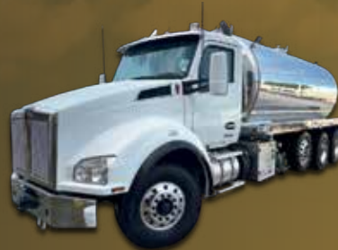
2025 KENWORTH T880 , CUMMINS ISX 450 HP, ALLISON 4500 RDS AUTO. TRANSMISSION, 5200 ALUMINUM TANK, NVE 4310 BLOWER 940 CFM, 36" ALUM. TOOLBOX, 79K GVWR. PRICE $286K + FET
