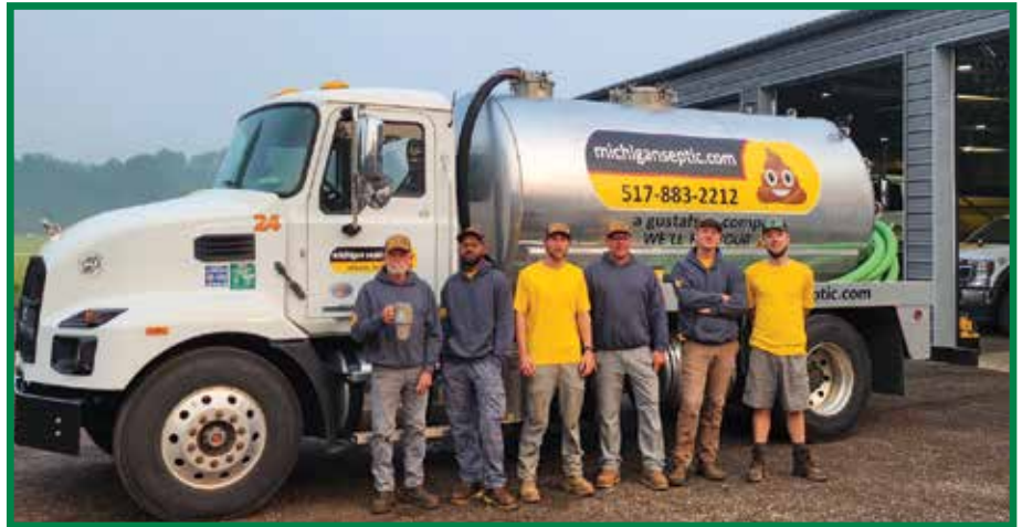
▲ The Michigan Septic team includes, from left, Roger Gustafson, Trae Smith, Cole Sworden, Matt Gustafson, Ethan Gustafson and Casey Fiedler. Behind them is a 2022 Mack MD6 with a 2,500-gallon aluminum tank and National Vacuum Equipment VE blower.
