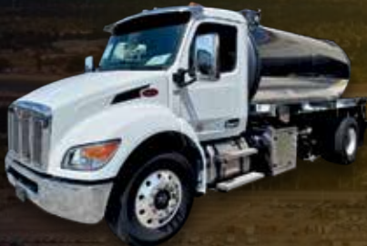
2025 PETERBILT 537 , CUMMINS ISB 300 HP, ALLISON 3000 RDS AUTO. TRANSMISSION, 2500 CARBON STEEL TANK, NVE 4310 BLOWER 940 CFM, 36" ALUM. TOOLBOX, 33K CVWR. CALL FOR PRICE
