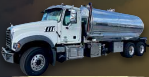
2024 MACK GRANITE , MP8 ENGINE 455 HP, 4500 RDS, ALLISON AUTOMATIC TRANSMISSION, 4200 ALUMINUM TANK, NVE BLOWER 940 CFM, 36" ALUMINUM TOOLBOX, 66K GVWR. PRICE $241K + FET
