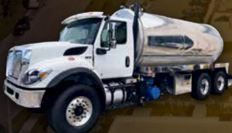
2025 INTERNATIONAL HV607 , CUMMINS ISL 350 HP., ALLISON AUTOMATIC TRANSMISSION, 4200 ALUMINUM TANK, FRUITLAND PUMP 510 CFM, 36" ALUMINUM TOOLBOX, 60K GVWR. PRICE $180K + FET
