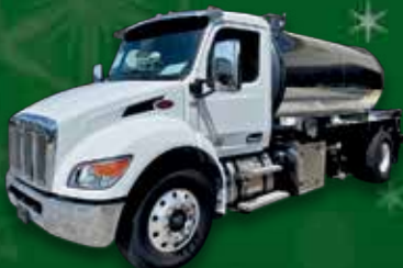
2024 PETERBILT 537 , 300 HP, CUMMINS ISB, 3000 RDS AUTO TRANS., DIFF LOCKS, AIR RIDE REARS, 2500 CS TANK, NVE 4310 BLOWER 940 CFM, 36" TOOLBOX, TOW HITCH, CHROME PACKAGE. CALL FOR PRICE
