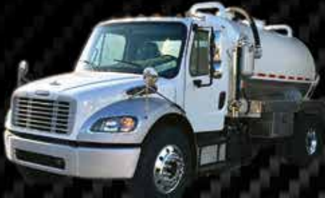
2024 Freightliner M2 - 2,000 Gal., Allison Automatic Trans., Cummins ISB, 250 H.P., A/C, C/C, Jake Brake, Big Pump NVE 607, 380 CFM, 26,000 GVW - No CDL - $140,000
