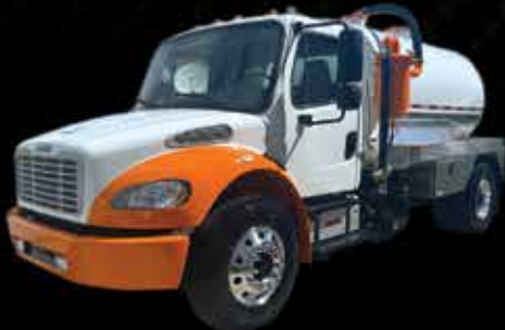
2024 Freightliner M2 - 2,000 Gal., Allison Automatic Trans., Cummins ISB 250 H.P., A/C, C/C, Jake Brake, Big Pump NVE 607, 380 CFM, 26,000 GVW - No CDL - $140,000
