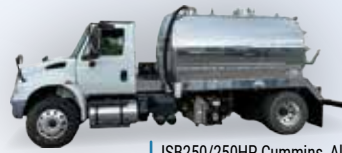
2015 International 4300 | ISB250/250HP Cummins, Allison 2500 RDS, 12/21, 2,650 gallon aluminum tank, NVE 607 package
