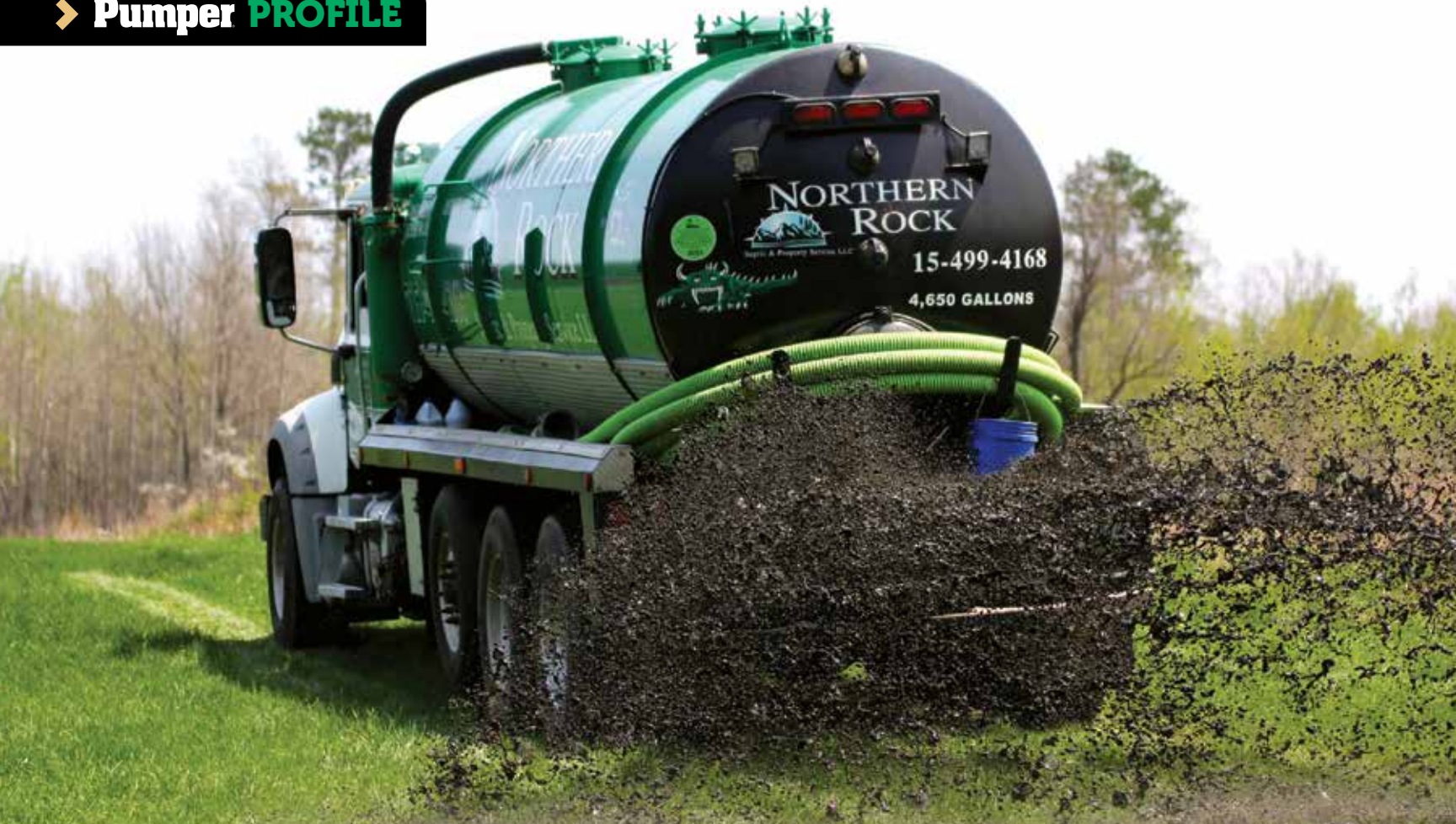
► The crew at Northern Rock land-applies septage in a field near the office whenever possible to minimize disposal costs at the local wastewater treatment plant.
