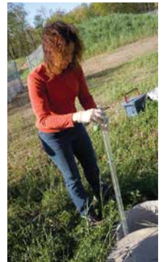
▲ Sara Heger uses a Sludge Judge to produce a core sample.
