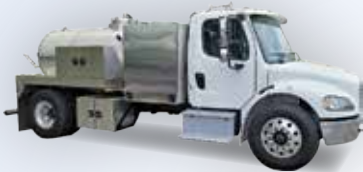
2023 Freightliner | NVE 607, Heated ProVac cabinet, 950 SS tank GREASE TRUCK | NON-CDL
