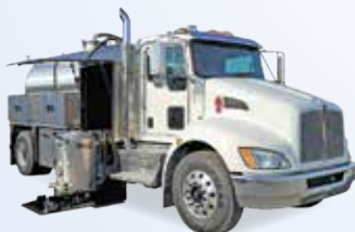
2015 International 4300 | ISB250/250HP Cummins, Allison 2500 IN PRODUCTION | RDS, 12/21, 2,650 gallon aluminum tank, NVE 607 or B500 package
