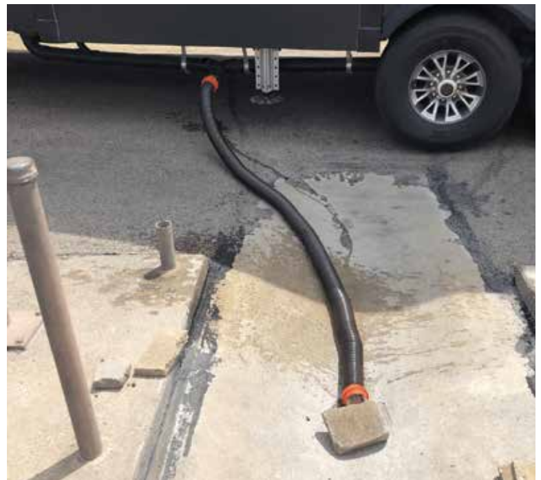
▲ At a campground dumpsite, the drain hose is connected to the outlet of the RV holding tank.
