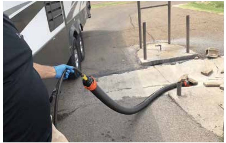
▲ A camper rinses out the drain hose after emptying the RV holding tank.
