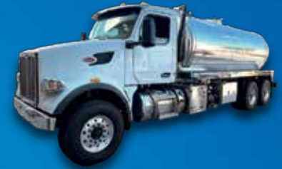
2024 PETERBILT 567 , CUMMINS ISX 450 HP, ALLISON AUTOMATIC TRANSMISSION, 4200 ALUMINUM TANK, NVE 4310 BLOWER 940 CFM, 36" TOOLBOX, CHROME PACKAGE. CALL FOR PRICE
