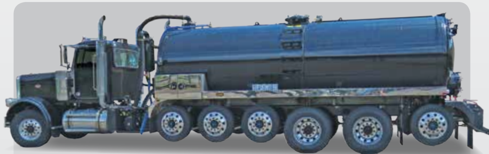
5500 Gallon Stainless Steel Tank ◊ NVE 4307 Blower
