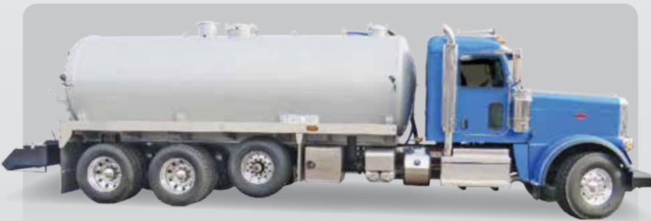
5000 Gallon Carbon Steel Tank ◊ 607 NVE Pump
