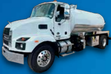
2024 MACK MD7 , 300 HP, CUMMINS ISB, 3000 RDS AUTO TRANS., DIFF LOCKS, AIR RIDE READ, 2500 CARBON STEEL TANK, NVE BLOWER 426 CFM, 36" TOOLBOX, CHROME PACKAGE. CALL FOR PRICE
