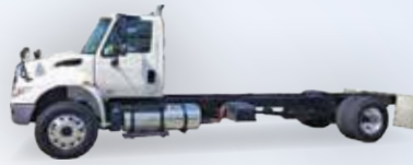
2015 International 4300 IN PRODUCTION | ISB250/250HP Cummins, Allison 2500 RDS, 12/21, 2,650 gallon aluminum tank, NVE 607 or B500 package
