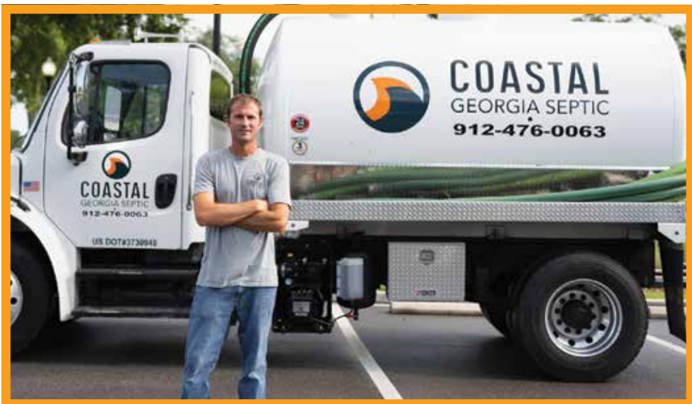
▲ Gavin Earl's truck is a Freightliner with a 2,500-gallon tank and a National Vacuum Equipment pump.
