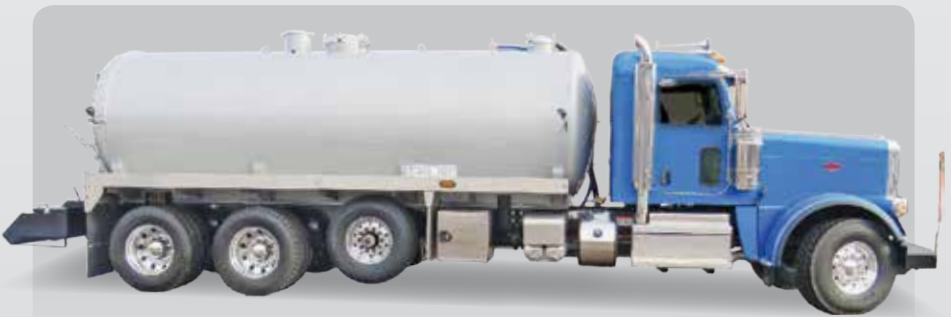
5000 Gallon Carbon Steel Tank ◊ 607 NVE Pump
