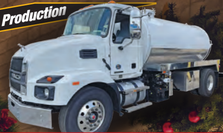
2024 Mack MD7, 300 hp, Cummins ISB, 3000 RDS auto trans., diff locks, air ride rear. 2500 CS Tank, NVE blower 426 cfm, 36" toolbox, Chrome package. Call For Price
