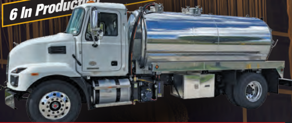
2024 Mack MD7, 300 hp, Cummins ISB, 3000 RDS auto trans., diff locks, air ride rear. 2500 alum tank, Masport Titan 407 cfm, 36" toolbox, Chrome package. Call For Price
