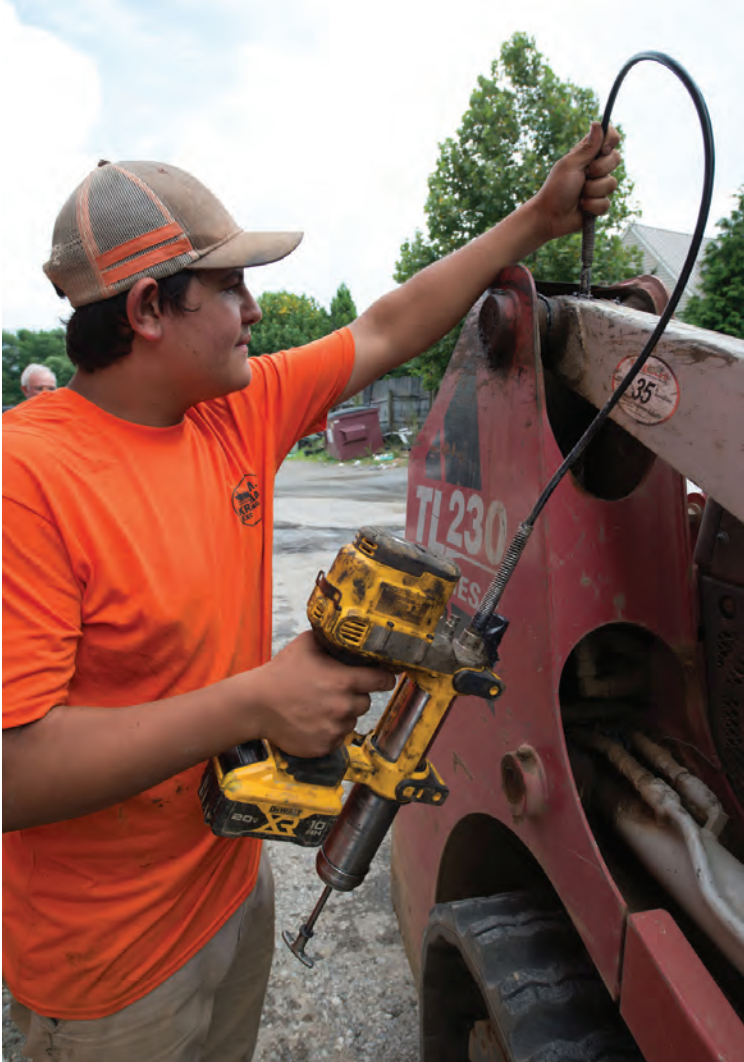
◀ Romero hits grease fittings on a Takeuchi skid loader during a maintenance check.
