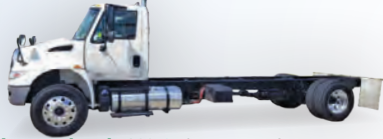
2015 International 4300 IN PRODUCTION | ISB250/250HP Cummins, Allison 2500 RDS, 12/21, 2,650 gallon aluminum tank, NVE 607 or B500 package
