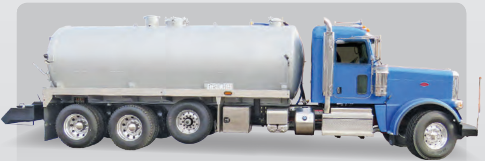
5000 Gallon Carbon Steel Tank ◊ 607 NVE Pump
