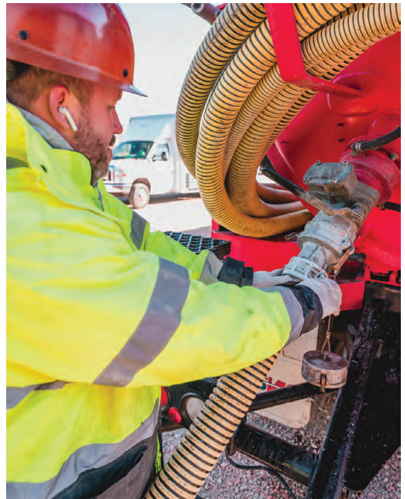
▲ After completing a septic pumping job, Matt Bunce disconnects the hose from the vacuum truck.
