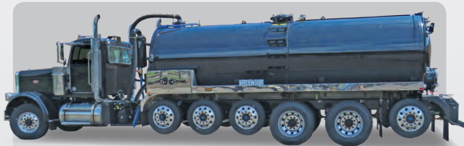
5500 Gallon Stainless Steel Tank ◊ NVE 4307 Blower
