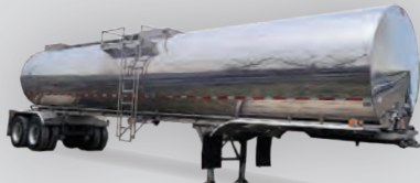
2018 9000 Gallon | 93,000 GVWR transport (aluminum tank Tandem Trailer | insulated stainless steel wrapped) 6" discharge
