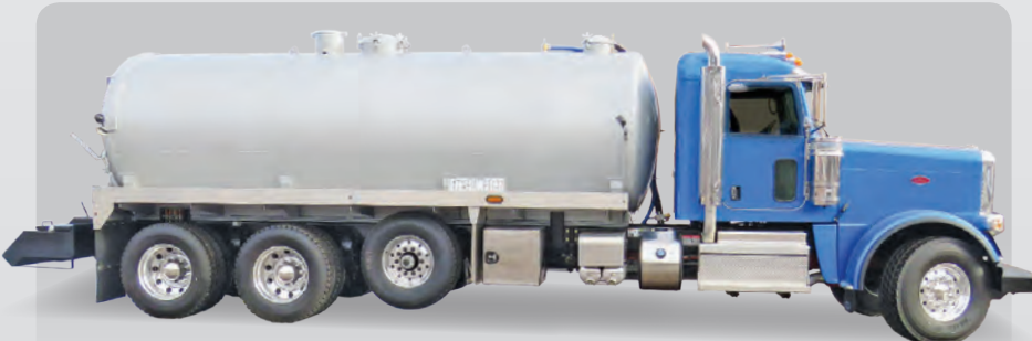
5000 Gallon Carbon Steel Tank ♦ 607 NVE Pump
