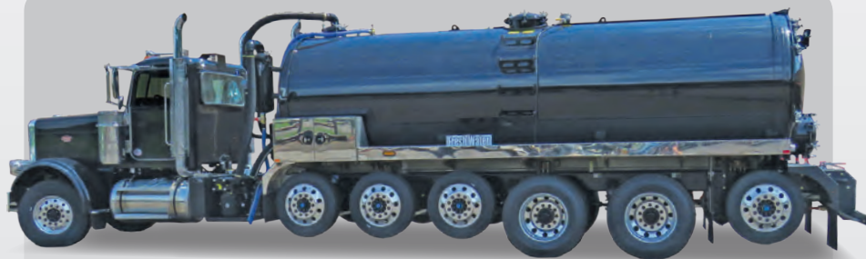
5500 Gallon Stainless Steel Tank ♦ NVE 4307 Blower
