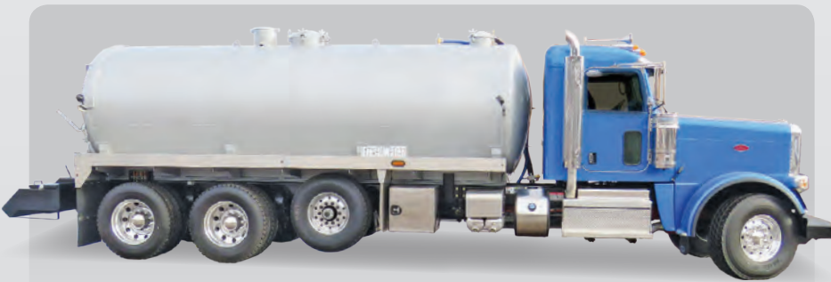
5000 Gallon Carbon Steel Tank ◊ 607 NVE Pump
