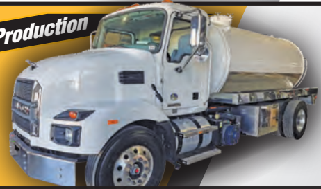
2023 Mack MD7, 300 hp, Cummins, Allison auto, chrome bumper and grille, 2500 CS tank, Masport Titan 407 cfm, diff locks, air ride rear. Call for Price
