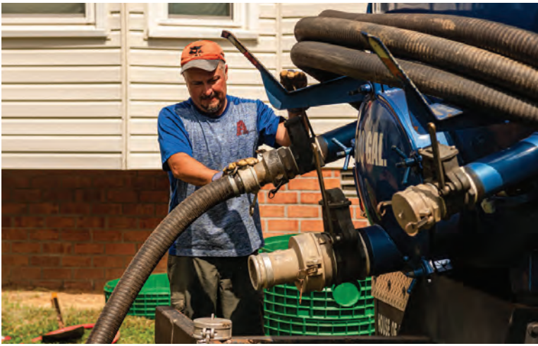
Ernie Anderson connects a septic hose to the rear of the truck.
