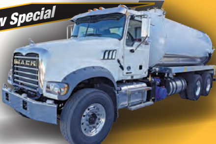
2023 Mack Granite MP8, 455 hp. Allison 4500 Rrds, 4200 CS tank, Fruitland pump, 530 cfm. *201K Plus FET
