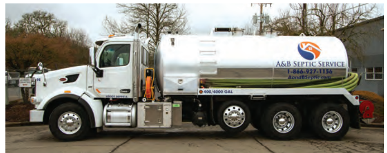
A&B Septic Service runs this 2021 Peterbilt 567 built out by Imperial Industries with a 4,200-gallon stainless steel tank and National Vacuum Equipment pump.
