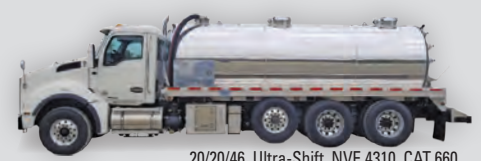
2023 Kenworth T880 | 20/20/46, Ultra-Shift, NVE 4310, CAT 660 jetter package, LED lights, LED strobes, 4-camera package, NAV system, alum. tank CALL FOR PRICING
