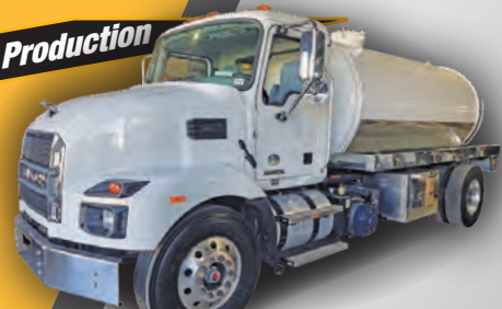
2023 Mack MD7, 300 hp. Cummins, Allison auto, chrome bumper and grille, 2500 CS tank, Masport Titan 407 cfm, diff locks, air ride rear. $126K
