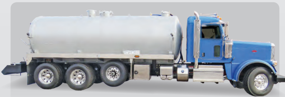
5000 Gallon Carbon Steel Tank ◊ 607 NVE Pump
