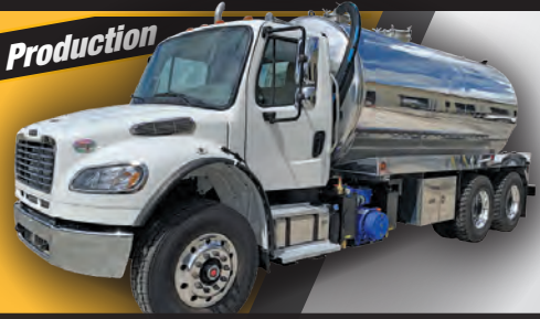
2022 Freightliner M2, Cummins 350 hp, auto, 4200 alum tank, Fruitland 530 cfm pump, 36" alum. toolbox. *169K plus FET
