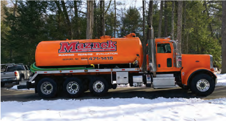
📍 This is Maznek's 2015 Peterbilt vacuum truck from Pik Rite with a 4,600-gallon steel tank and Masport pump.
