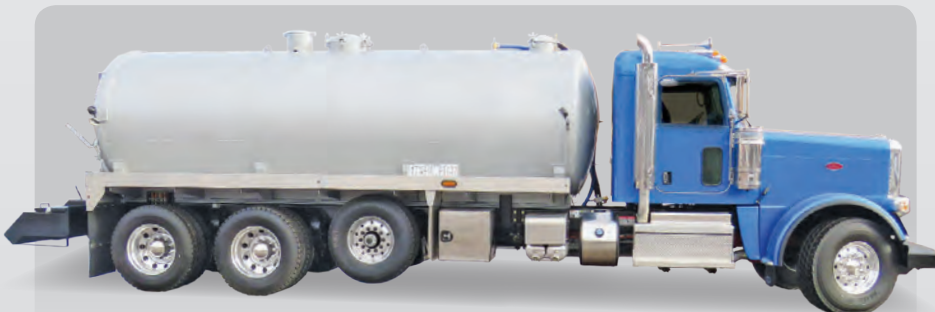
5000 Gallon Carbon Steel Tank ◊ 607 NVE Pump
