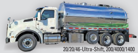
20/20/46-Ultra-Shift, 200/4000/1400 aluminum decant tank, NVE 4310 blower package, strobes, cameras 2021 Kenworth T880 CALL FOR PRICING
