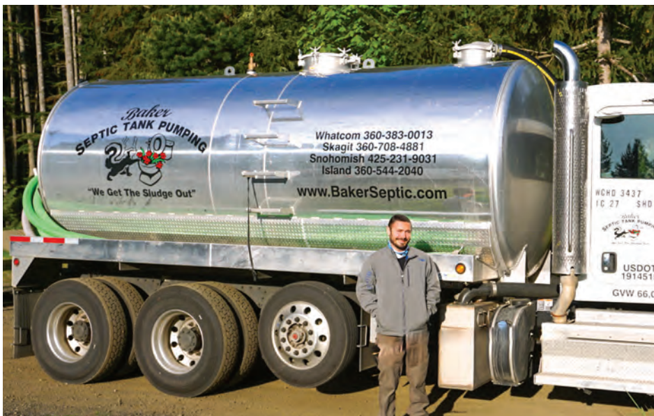
Justin Wells and a 2021 Peterbilt with a FlowMark Vacuum Trucks 4,200-gallon aluminum tank and National Vacuum Equipment 900 cfm blower.
