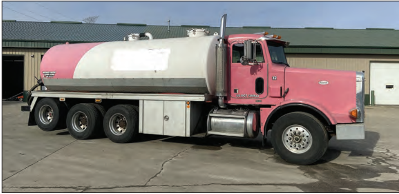
1998 Peterbilt 378, 4000 Gallon Steel Tank, 485K Mi., C-10 — 385 HP, 8LL, All Alum. Wheels, Newer Tag Axle, 18,000FA/40,000RA, Air Ride Susp., Wheel Lock, NVE Pump - 4 Yrs. Old.
