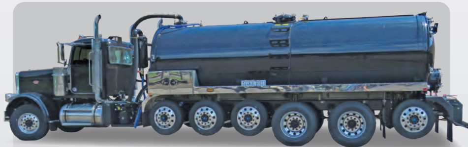
5500 Gallon Stainless Steel Tank ◊ NVE 4307 Blower
