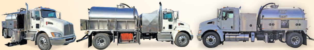
2021 T370 Kenworth GREASE TRUCK | 300HP, Allison Auto, 33,000 G.V.W.R) 1800 gallon stainless steel (ITI) tank, NVE 607 ProMax package, heat collars (heat through tank), heated cabinet for ProVac unit w/hydraulic lift, Hannay hose reel w/100' 2" hose in heated cabinet.
