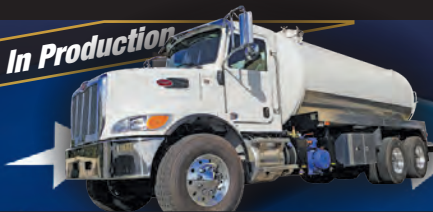
2022 Peterbilt 348, Cummins 350 hp, 10 spd, 4000 carbon steel tank, Fruitland 510 cfm, chrome package. $147,126 Plus FET
