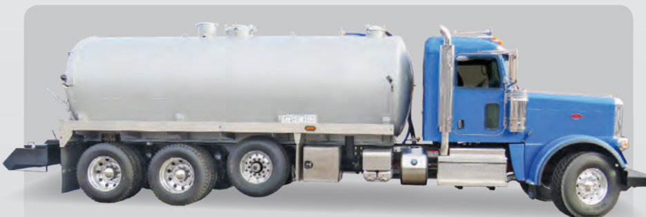
5000 Gallon Carbon Steel Tank ◊ 607 NVE Pump
