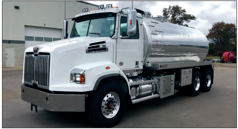
2022 4700SB , L9-360 HP, 3000RDS Allison Auto., 18K FA/40K RA, 4,000 Gallon Alum. Tank, All Alum. Wheels, Available w/4307 or 4310 NVE Blowers. Units also Available w/4200 or 5000-Gal. Set-Ups.
