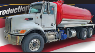
2022 Peterbilt 348, Cummins 350 hp, 10 spd manual, 4000 carbon steel tank, Fruitland pump 510 cfm. *148,126 Plus FET
