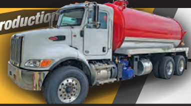
2022 Peterbilt 348, Cummins 350 hp, 10 spd manual, 4000 carbon steel tank, Fruitland pump 510 cfm. *145,500 Plus FET
