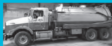
2011 Kenworth T800 , Cummins ISX 485, 18-speed, Transway-built 4,000-gallon waste, 200-gallon freshwater with 10 gpm 3,000 psi jetter. Full hoist, vibrator and rear-open door. Transway 1200 pump. 167,500 miles, 14,500 hours. Asking $100,000. 802-658-6243. dispatch@pandseptic.com. VT (P06)
