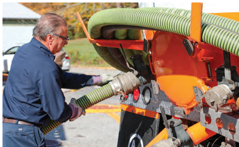
Parent connects a suction hose to his pump truck at a commercial pumping location.
