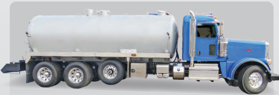
5000 Gallon Carbon Steel Tank ◊ 607 NVE Pump
