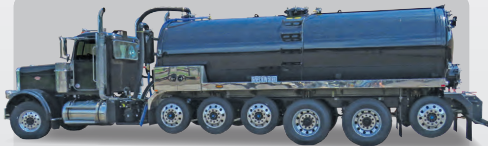
5500 Gallon Stainless Steel Tank ♦ NVE 4307 Blower
