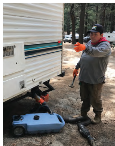
Each rental RV comes with a rolling 10-gallon "blue boy" tank for graywater. Angel Talamantes is shown pumping the auxiliary tank.
