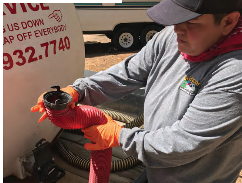
👉 Angel Talamantes shows the red Valterra hose that runs between the tank-mounted vacuum hose and the adaptor to connect to the RV dump valve.
