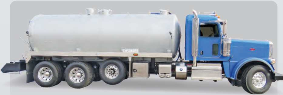
5000 Gallon Carbon Steel Tank ♦ 607 NVE Pump
