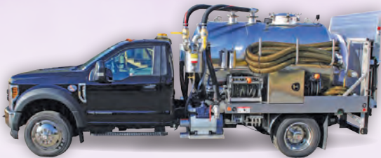
GH1200 800 waste 400 water with Masport HXL4 and Udor high pressure wash down pump
