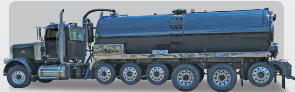
5500 Gallon Stainless Steel Tank ◊ NVE 4307 Blower
