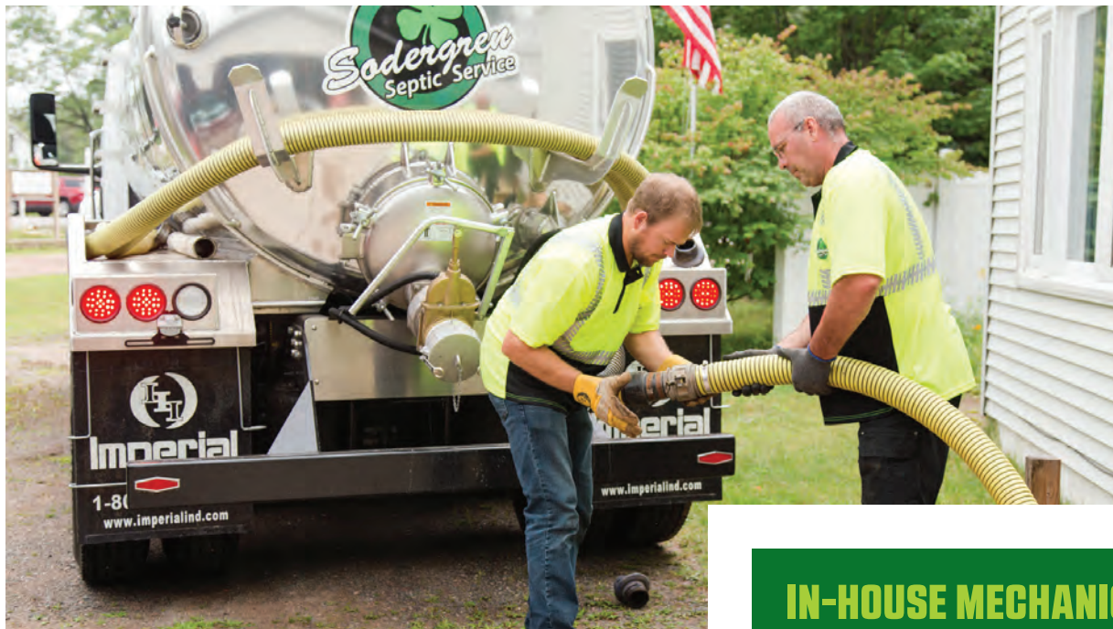
Left: Carey and Farkas link hoses to reach a tank on a residential call. The service truck is from Imperial Industries and carries a Fruitland pump.
