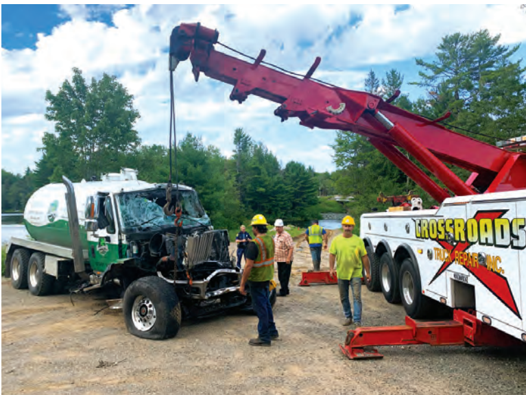
Left: The truck itself was a total loss, but the wastewater tank was undamaged and will be reused.
