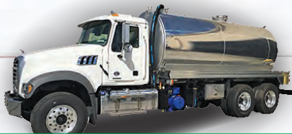
2020 Mack MHD. Chrome package, Cummins 350 hp, Jake brakes, Allison auto trans., 4200 gal. alum tank, Fruitland 510 cfm pump, 60K GVW. *158,500 Plus FET
