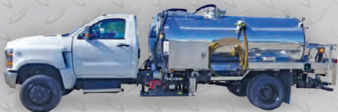
2019 Chevy 5500 | 4 x 4, diesel 1500 RVT, NVE 304 engine package. CALL FOR PRICING
