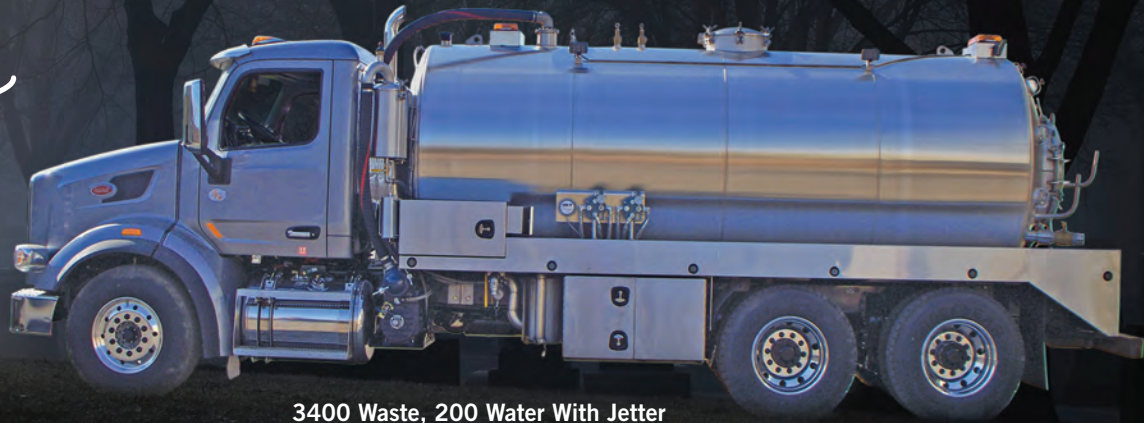
3400 Waste, 200 Water With Jetter
