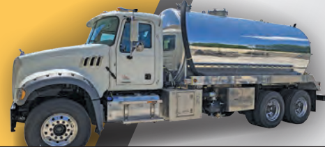
2020 Mack Granite, MP8-455 hp, Allison 4500 RDS, 4000/200 alum. NVE 940 cfm blower, 10 gpm jetter. $213,885 Plus FET • In Stock!
