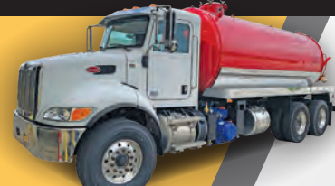
2021 Peterbilt 348, Cummins 350 hp, 10 spd manual, 4000 carbon steel tank, Fruitland pump 510 cfm. $140,700 Plus FET • In Production!
