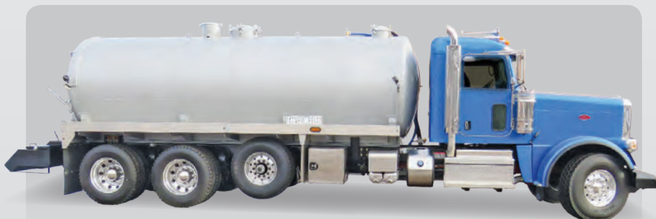
5000 Gallon Carbon Steel Tank ◆ 607 NVE Pump
