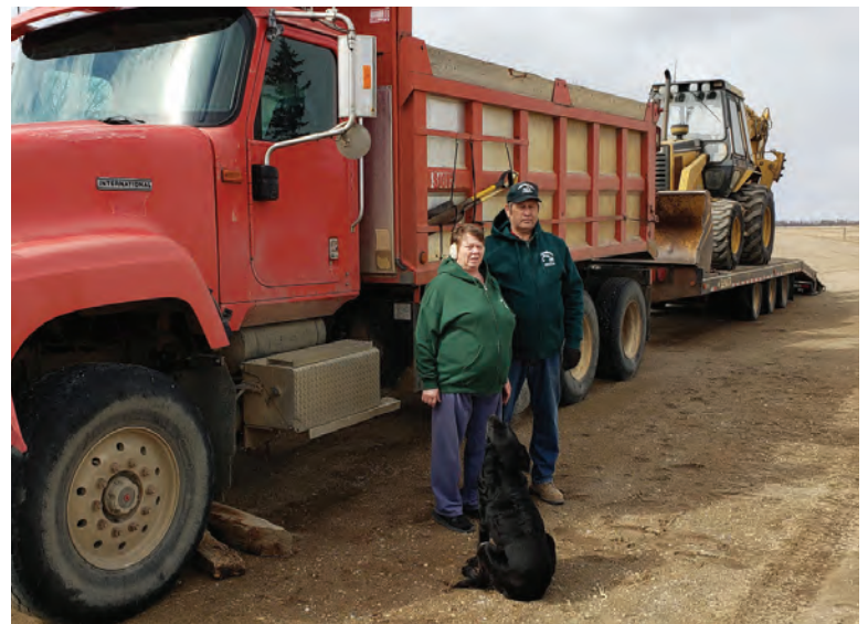
Above: Tom and Peggy Schimelfenig stand by a 2000 International 5500I tri-axle dump truck with a 16-foot Ox Bodies insulated box, a 2002 Felling Trailers FT-50-3 trailer and a 1998 Caterpillar 446B loader backhoe (as well as Casey the dog).
