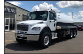
2020 M2-106 , 350 HP Cummins, Automatic, Air Ride with 3600 Gal Imperial Tank.
