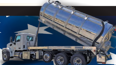
2020 Peterbilt 567, Cummins ISX 450 hp auto, 5000/200 alum. hoist tank, NVE 940 cfm blower, 10 GPM@3000 PSI hydraulic jetter, internal spray heads for easy tank cleaning, backup camera, 37" traffic advisor, two rear 30" slanted top lid tool boxes. $250,000 Plus FET • In Stock!
