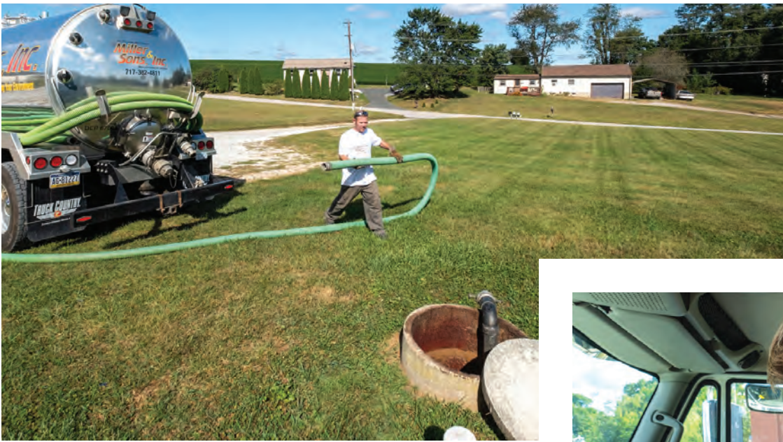
Left: Jared Miller pulls hose to reach a septic tank. The truck is 2019 Freightliner from Imperial Industries and carrying a National Vacuum Equipment 4307 pump.
