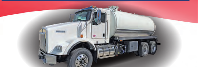
2021 Kenworth T800, Cummins ISX 450 hp, 18 spd, 46K Hendrickson spring rears 4000 gal. carbon steel tank, 407 cfm pump. $175,000 Plus FET • In Production!
