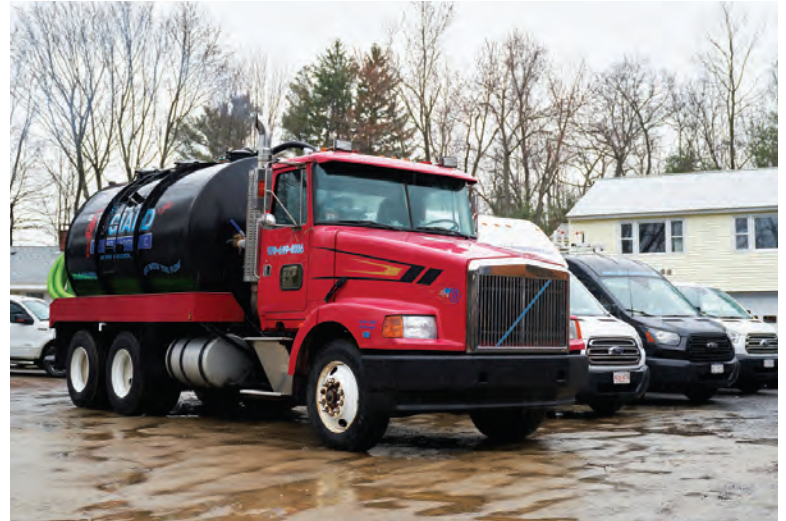
Below: The 1989 Volvo carries a new New England Mechanical Overlay tank and National Vacuum Equipment vacuum pump. It is shown with several plumbing Ford Transit and Transit Connect service vans used on the plumbing side of the business.
