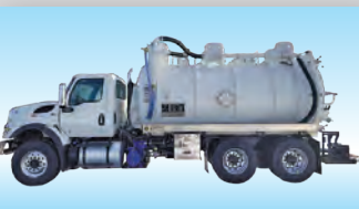
2020 Int'l HV607 Cummins LP, 370 HP 6 Spd Allison Trans., ASME 407/412 3200 gallon DOT Tank
