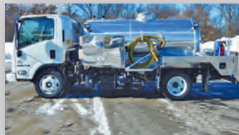
2020 Isuzu NRR NEW Isuzu NRR, 5.2L Isuzu Diesel, Auto Trans., 1300 Gal. Alum Tank, 900 Waste/400 Water, Masport HXL4V Vacuum Pump
