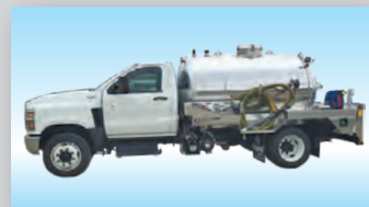
2020 Int'l CV515 Int'l 6.6 V8, 350 HP, 6 Spd Allison Auto Trans., 1300 Gal. Aluminum Tank, 900 Waste/400 Water, NVE304 Vacuum Pump
