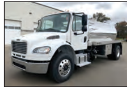
2020 Freightliner M2 106 , 300HP Cummins L9, Allison Auto, Air Ride, Diff Lock, 2500 Gal. Imperial Tank with NVE 607 Pump.
