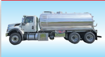
2020 Int'l HV 607 Cummins L9, 370 HP, Allison or 10 Spd Trans., 4000 Gal. Alum Imperial Tank, NVE Blower or Vane Pump
