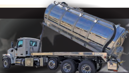
2020 Peterbilt 567, Cummins ISX 450 hp auto, 5000/200 Alum. hoist tank, NVE 940 cfm blower, 10 GPM@3000 PSI hydraulic jetter, internal spray heads for easy tank cleaning, backup camera, 37" traffic advisor, two rear 30" slanted top lid tool boxes. $250,000 Plus FET
