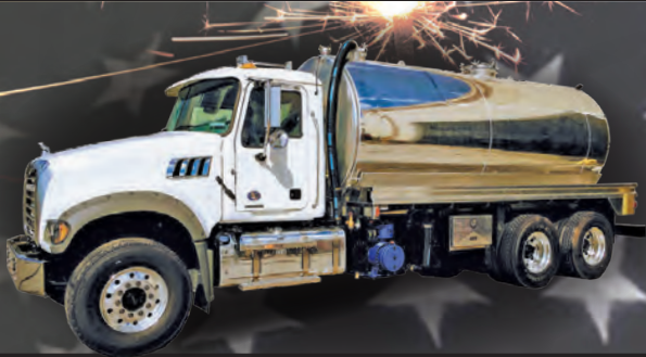
2020 Mack Granite MP8, 455 hp, Allison auto, 4000/200 alum. tank, Fruitland 512 cfm pump, Advance 5 gpm Jetter @ 3500 PSI. $196,000 Plus FET
