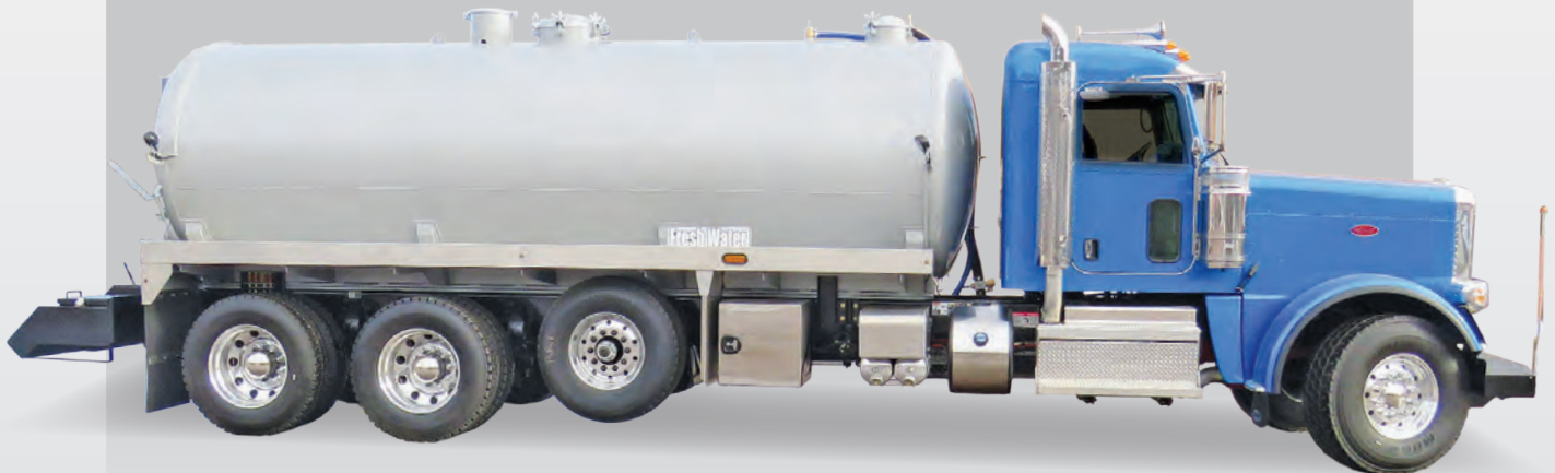
5000 Gallon Carbon Steel Tank ◊ 607 NVE Pump
