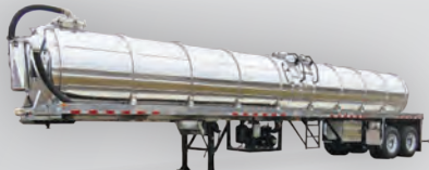
2020 7,000 Gallon Vacuum Trailer | Air suspension, NVE 887 pump package
