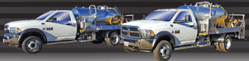
GH1100 800 waste/ 300 water mounted on a Dodge 5500
