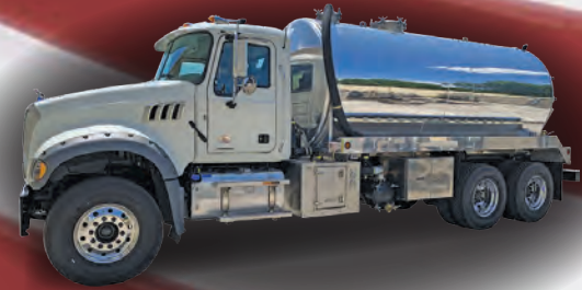
2020 Mack Granite, MP8-455 hp, Allison 4500 RDS, 4000/200 alum. NVE 940 cfm blower, 10 gpm jetter. $213,885 Plus FET • In Stock!
