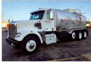
2012 122SD, DD15, 18-Spd, Full Lockers 4620 GAL Aluminum Tank with a Berkley Pump.
