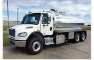
2020 M2106 350HP Cummins, Allison Automatic, Full Lockers, Air Ride, 4000GAL Alum., 4307 Blower.
