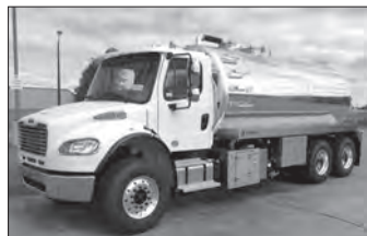
2020 M2 106, 350 HP Cummins, Allison Auto., 4000 Gal Aluminum, NVE4310 Blower, Multiple Available.
