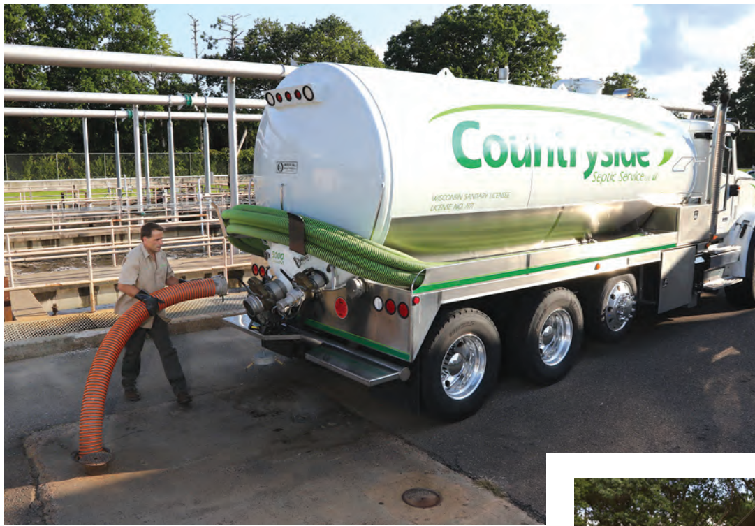
Left: Tom Jakubowicz makes a disposal run at the Chippewa Falls, Wisconsin, wastewater treatment plant. The 5,000-gallon tank on his new truck from Imperial Industries allows him to pump more tanks between trips to the dump station.
