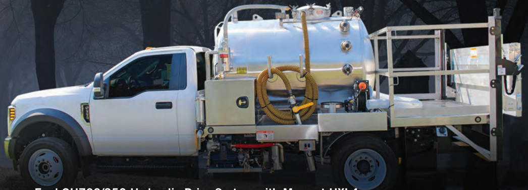
Ford GH700/350 Hydraulic Drive System with Masport HXL4
