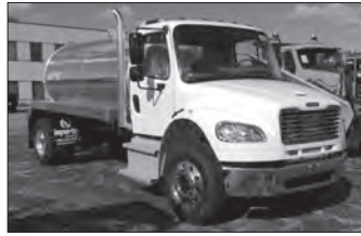
2020 M2106 , 300HP Cummins, Allison Automatic, 1760 Gal Aluminum and 1900 Stainless Steel Portable Service Trucks
