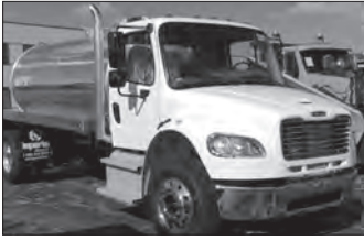
2020 M2 106 , 300HP Cummins L9, Allison Auto, Air Ride, Diff Lock, 2500 Gal. Imperial Tank with NVE 607 Pump
