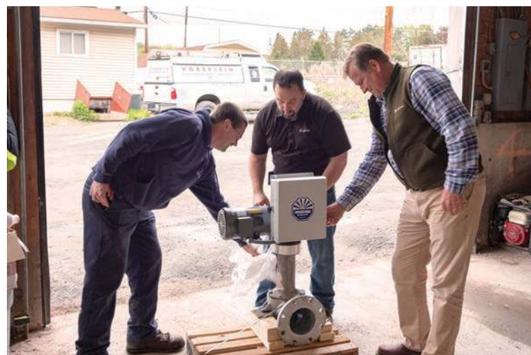
Mohrmann (left), Mike Sprague and Chris Ravenscroft inspect a Purestream comminutor prior to installation.
