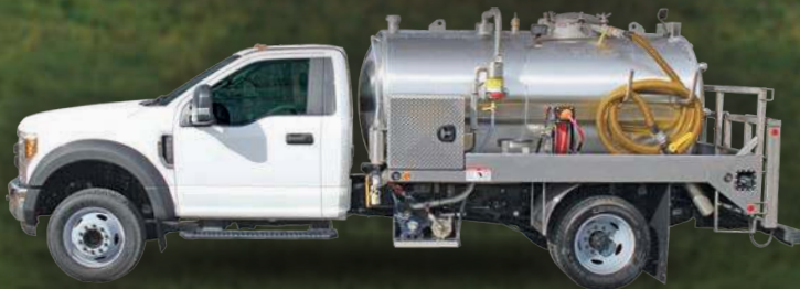
GH 800/300 Angle Drive Sys. Equipped with Masport HXL4, Dual Side Suction and MTH DC10 Wash Down Pump and Hose. Built Out of 304L Stainless Steel. Mounted on Ford F-550 4 x 2 Gas.
