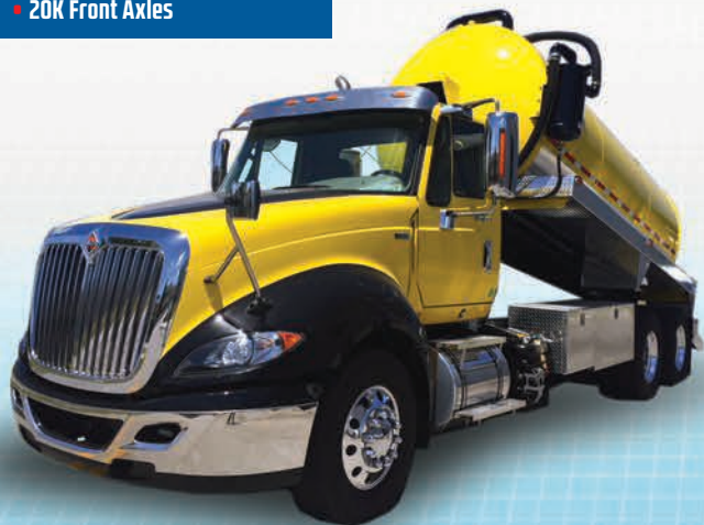
2011 International Prostar 4,000 Gal., Cummins ISX, 450 h.p., 10 spd. Full Hydraulic Dump
