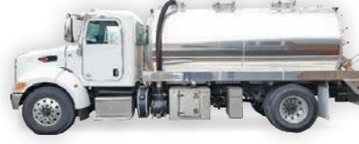
2019 Peterbilt 337 | 330HP, auto, 2800 gal. aluminum tank, NEW | NVE 4310 blower package.
