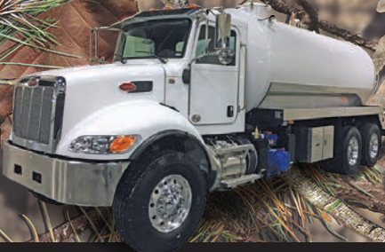
2020 Peterbilt 348 , Cummins 350 hp, 10 spd, chrome package, 4000 gal. carbon steel tank, 530 cfm pump. $137,500 Plus FET
