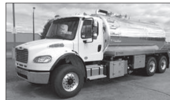
2019 M2106 with 4000 Gal. Tank , 350 HP Allison Automatic, Air Ride, Full Lockers, 4000 Gal. Aluminum NVE 4307 Blowers.
