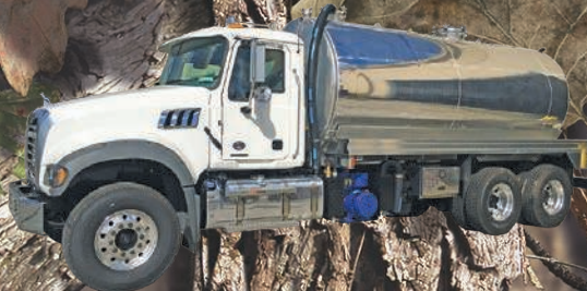
2019 Mack Granite, MP8 455 hp, Allison RDS 4500, 20K FA, 46k rears, 4200 alum. tank, choice big pump or blower
