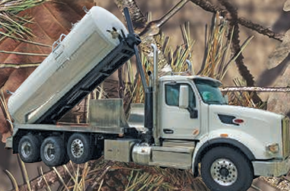
2020 Peterbilt 567, Cummins ISX 450 hp, Allison auto trans. 5000 gal. steel hoist or alum. tank, NVE 940 cfm blower, 12 gpm jetter w/ 200 gal. water tanks
