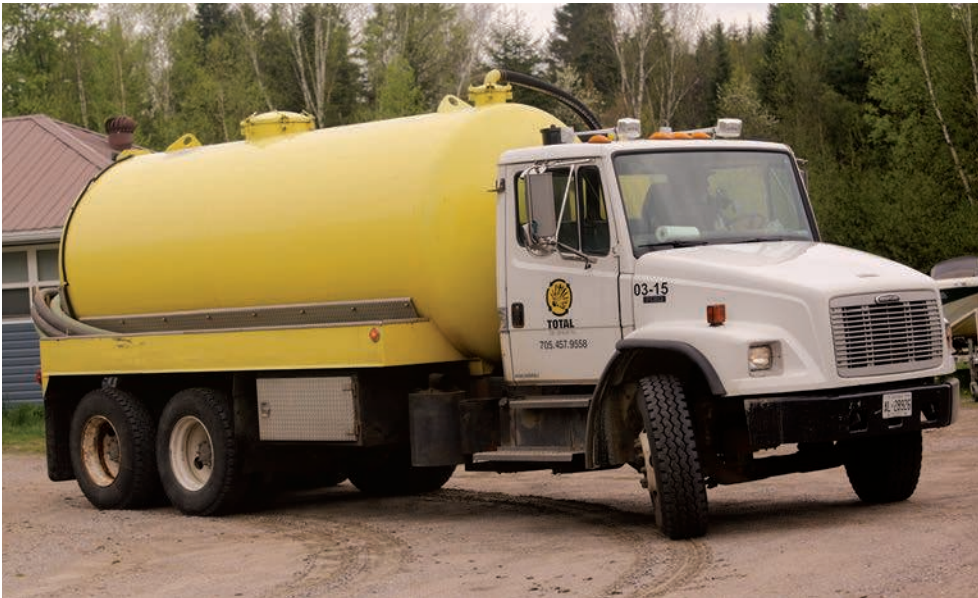
Left: One of two pumping rigs used by Total Site Services to pump septic tanks in rural Ontario, built out by Vacutrux and carrying Elmira Machine Industries / Wallenstein Vacuum pumps.
