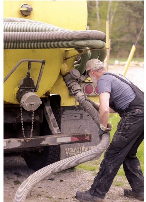
Below: Ben Ford attaches a suction hose to his pumping rig built out by Vacutrux and using a Elmira Machine Industries / Wallenstein Vacuum pump.
