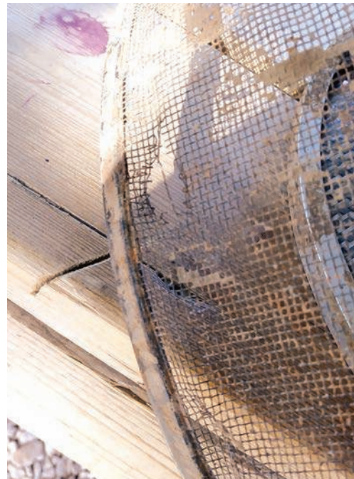
Joe Harp's face shield after he was hit by flying debris on a job site. The face shield prevented any major injuries from happening, but it did put a hole through the shield. (Photo courtesy of Joe Harp)
