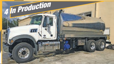
2019 Mack Granite ISL, Cummins 350 hp., Allison auto. - 4000 alum. tank, Fruitland high efficiency pump 512 CFM - FET not included. $153K
