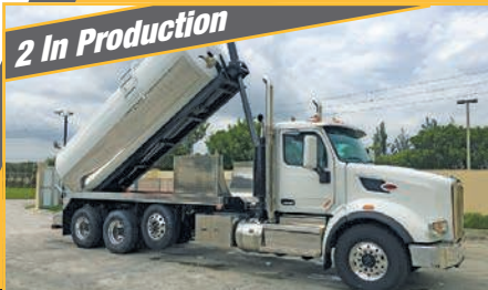
2020 Peterbilt 567, Cummins ISX 450 hp., Allison auto trans. 5000 gal. steel hoist or alum. tank, NVE 940 cfm blower, 12 gpm jetter w/ 200 gal. water tanks
