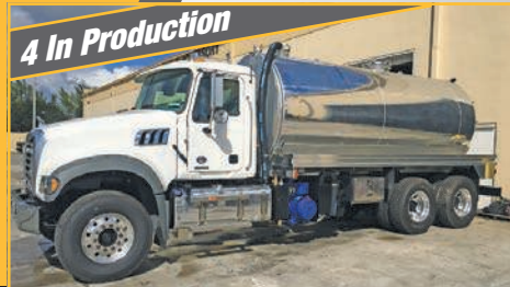
2019 Mack Granite ISL, Cummins 350 hp., Allison auto. - 4000 alum. tank, Fruitland high efficiency pump 512 CFM - FET not included. $153K
