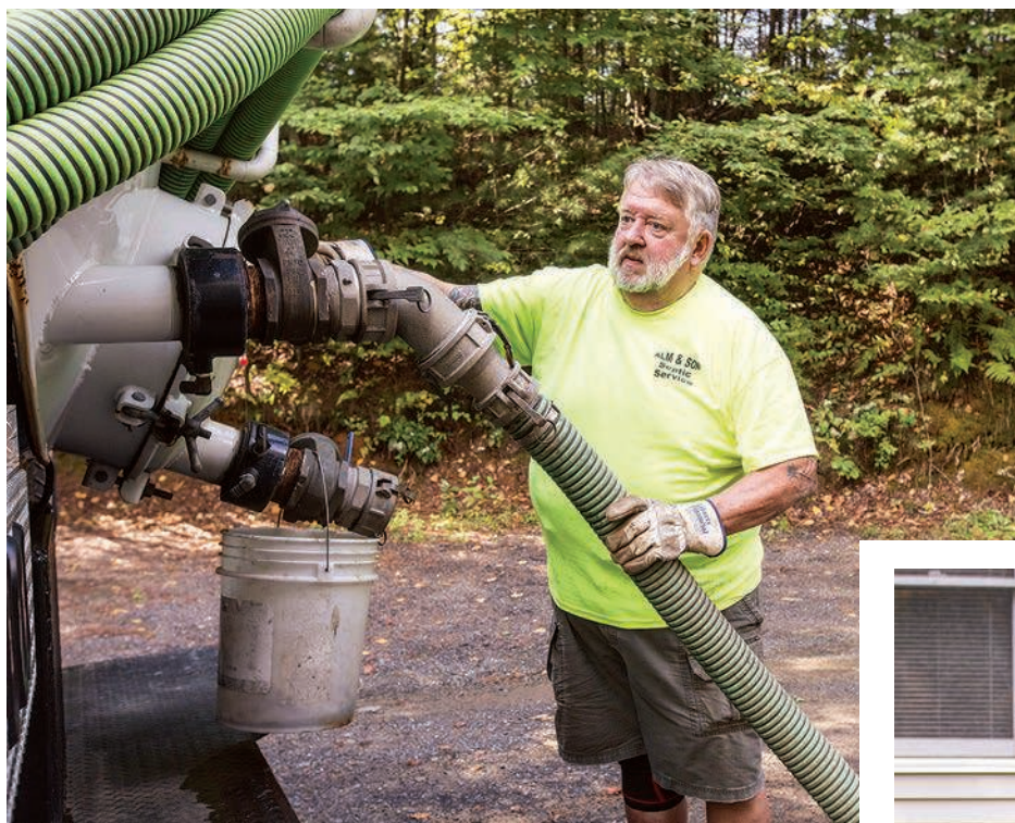
Left: During a service call, Karl Alm opens the suction valve on his truck outfitted by Osco Tank & Truck Sales with a 3,500-gallon steel tank and a National Vacuum Equipment Challenger pump.
