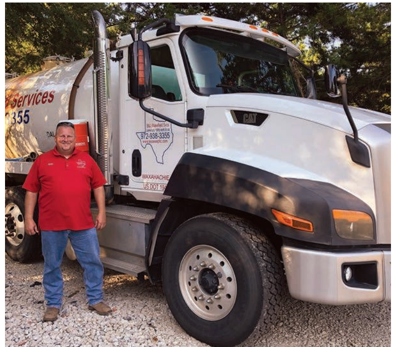
Brian Wakefield with a 2015 Caterpillar CT660 with a 3,600-gallon tank and Masport HXL400W.
