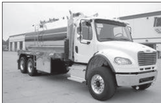
2014 M2-106, 350 HP - Cummins, 20# FA, Air Ride Suspension, 4000 Gal. Alum., 337755.
