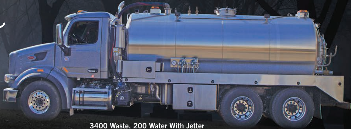
3400 Waste, 200 Water With Jetter
