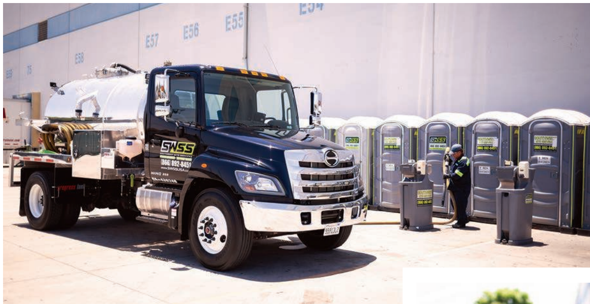
Left: Technician Carlos Rubalcava uses a Hino truck built out with a tank from Progress Tank and a pump from National Vacuum Equipment to clean PolyJohn restrooms and hand-wash stations.
